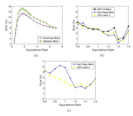
Fig. 4: Error comparison between  $\dot{q}$  using Eq. (5) results and the simulation using detailed chemical kinetics mechanisms,  $\dot{q}_{num}$ , as a function of the equivalence ratio: (a) H<sub>2</sub>/air mixtures (b) CH<sub>4</sub>/air mixtures (c) C<sub>3</sub>H<sub>8</sub> mixtures.
