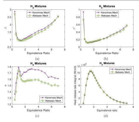
Fig. 5: Results for  $H_2$ /air mixtures with two different kinetics mechanism: Keromnes Mech ( $\diamond$ ) and Alekseev Mech ( $\times$ ). Behavior as a function of the equivalence ratio of (a) Zel'dovich number, (b)  $\beta'$  parameter, (c) n parameter, (d) Heat release rate normalization integral,  $I_q$ .
