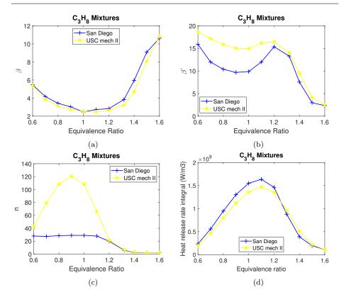
Fig. 7: Results for  $C_3H_8$ /air mixtures with two different kinetics mechanism: San Diego Mech (+) and USC Mech II (\*). Behavior as a function of the equivalence ratio of (a) Zel'dovich number,  $\beta$ , (b)  $\beta'$  parameter, (c) n parameter, (d) Heat release rate normalization integral,  $I_q$ .
