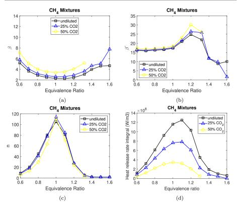
Fig. 8: Results for CH<sub>4</sub>/CO<sub>2</sub>/air mixtures as a function of the equivalence ratio. (a) Zel'dovich number,  $\beta$ , (b)  $\beta'$  parameter, (c) n parameter, (d) Heat release rate normalization integral,  $I_q$ .
