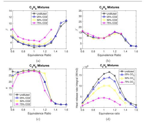
Fig. 9: Results for  $C_3H_8/CO_2/air$  mixtures as a function of the equivalence ratio. (a) Zel'dovich number,  $\beta$ , (b)  $\beta'$  parameter, (c) n parameter, (d) Heat release rate normalization integral,  $I_q$ .
