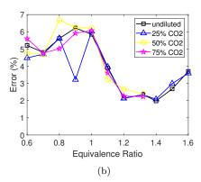
Fig. 10: Error comparison between the Eq. (5) results and the simulation using chemical kinetics mechanisms: (a)  $\rm CH_4/CO_2/air$  mixtures, (b)  $\rm C_3H_8/CO_2/air$  mixtures.
