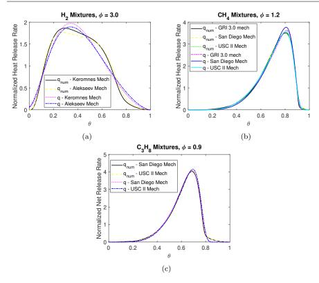
Fig. 3: Normalized heat release rate as a function of the progress variable comparison for the different kinetics mechanism used: (a)  $H_2$ /air mixture,  $\phi$ =3.0, (b)  $CH_4$ /air mixture,  $\phi$ =1.2 and (c)  $C_3H_8$ /air mixture,  $\phi$ =0.9.
