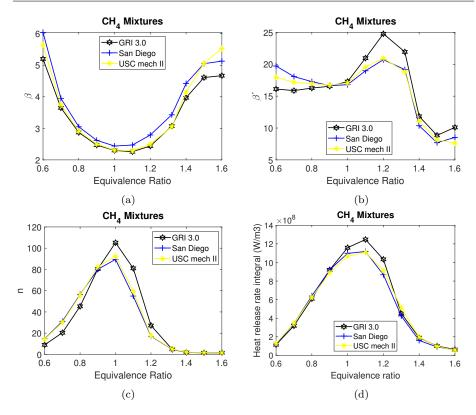
Fig. 6: Results for CH<sub>4</sub>/air mixtures with three different kinetics mechanisms: GRI 3.0 (hexagram), San Diego Mech (+) and USC Mech II (\*). Behavior as a function of the equivalence ratio of (a) Zel'dovich number,  $\beta$ , (b)  $\beta'$  parameter, (c) n parameter, (d) Heat release rate normalization integral,  $I_q$ .
