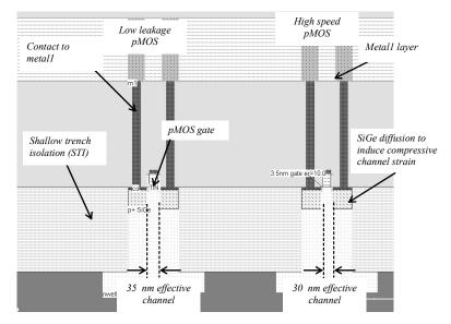
*Figure 10: Cross-section of the pMOS devices*
