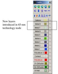
Figure 11: Microwind window with the palette of layers including 8 levels of metallization
