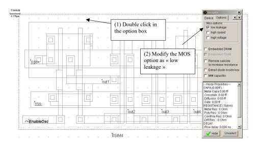
Figure 20: Changing the MOS option into low leakage mode
