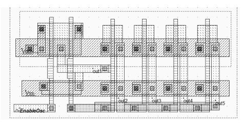
Figure 18 : The schematic diagram and layout of the ring oscillator used to compare the analog performances in high speed and low leakage mode (INV5Enable.MSK)
