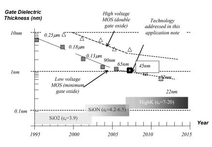
Figure 1 : The technology scale down towards nano-scale devices
