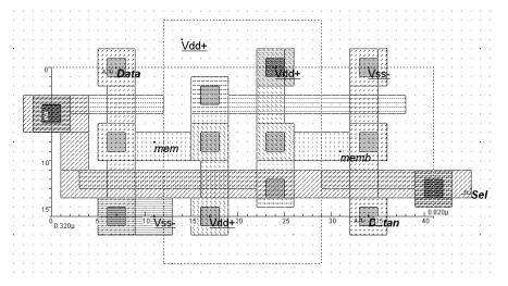
Figure 21: The 6-transistor RAM layout using 45-nm design rules (Ram6T 45nm.MSK)
