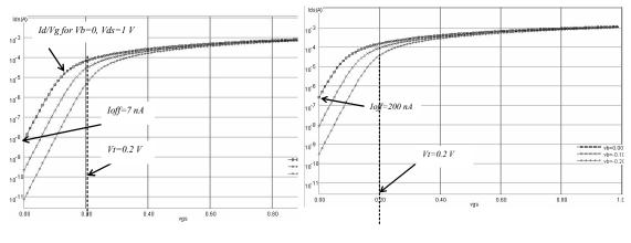
(a) low leakage MOS (Leff=35 nm) (b) high speed MOS (W=1 µm, Leff=30 nm)
