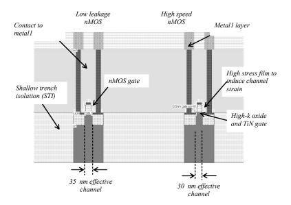
Figure 7: Cross-section of the nMOS devices (allMosDevices.MSK)
