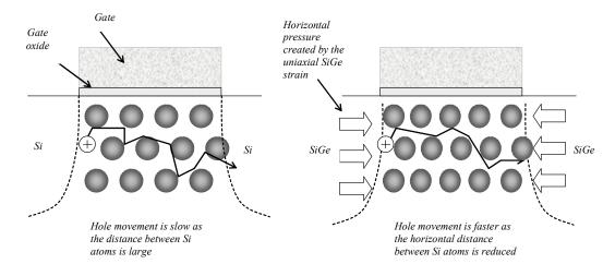
Figure 6: Compressive strain to reduce the distance between atoms underneath the gate, which speeds up the hole mobility of p-channel MOS devices
