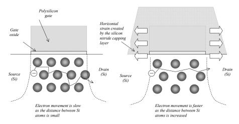
Figure 5: Strain generated by a silicon-nitride capping layer which increases the distance between atoms underneath the gate, which speeds up the electron mobility of n-channel MOS devices
