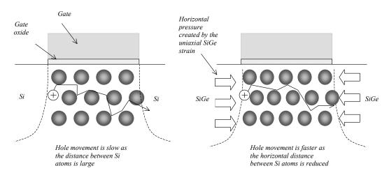
Figure 6: Compressive stain to reduce the distance between atoms underneath the gate, which speeds up the hole mobility of p-channel MOS devices
