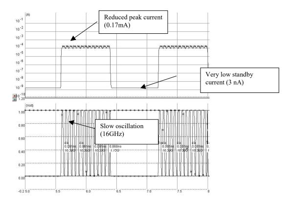
Figure 20: Simulation of the ring oscillator in low leakage mode. The oscillating frequency is slower but the standby current is very low (Inv5Enable.MSK)
