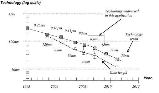
Figure 1: The technology scale down towards nano-scale devices
