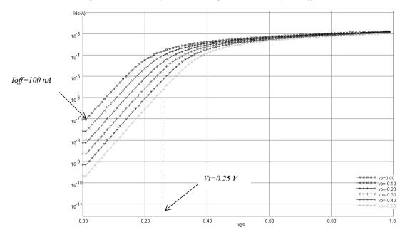
(b) Id/Vg characteristics for high speed MOS (W=1 \mu m, Leff=35 nm)
