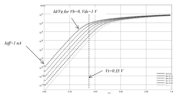
(a) Id/Vg characteristics for low leakage MOS (W=1 \mu m, Leff=50 nm)
