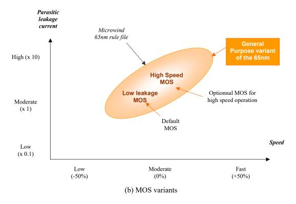
Figure 3: Introducing three variants of the 65nm technology(a), and two types of MOS within each variant (b)
