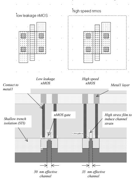
Figure 7: Cross-section of the nMOS devices (allMosDevices.MSK)
