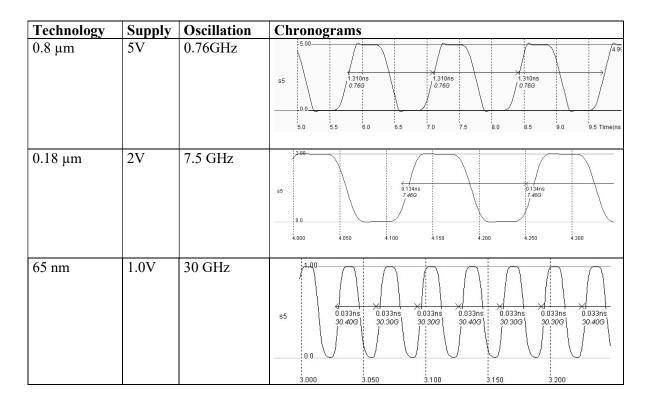
Figure 16: Oscillation frequency improvement with the technology scale down (Inv5.MSK)
