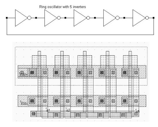
Figure 15: Schematic diagram and layout of the ring oscillator used for simulation (INV5.MSK)
