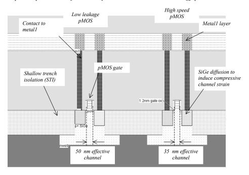
Figure 10: Cross-section of the pMOS devices
