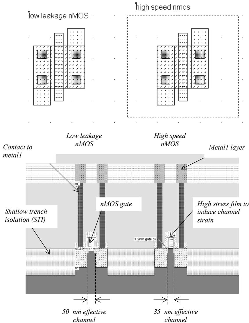
Figure 7: Cross-section of the nMOS devices (allMosDevices.MSK)
