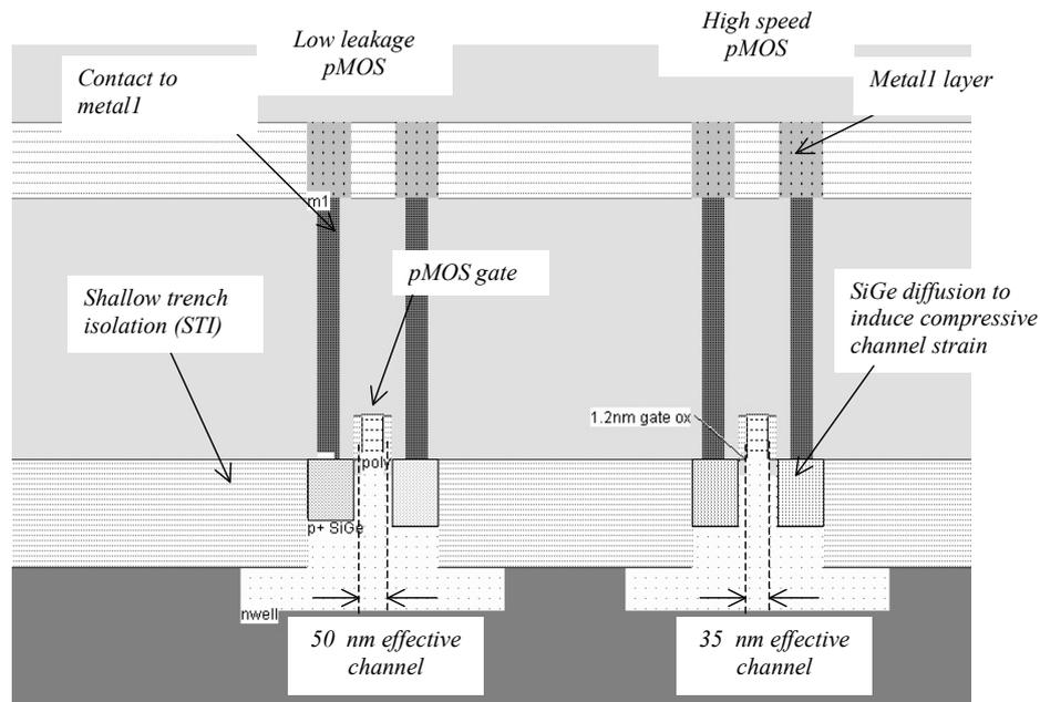
Figure 10: Cross-section of the pMOS devices
