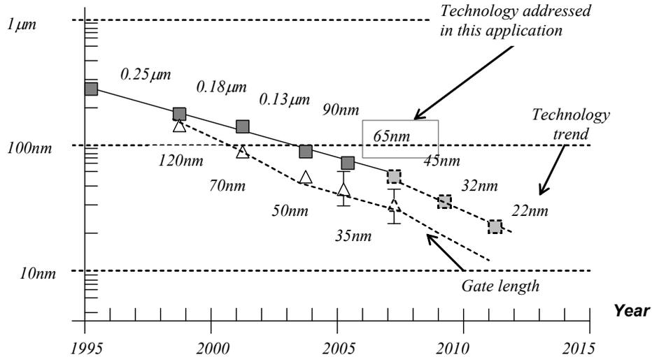
Figure 1 : The technology scale down towards nano-scale devices
