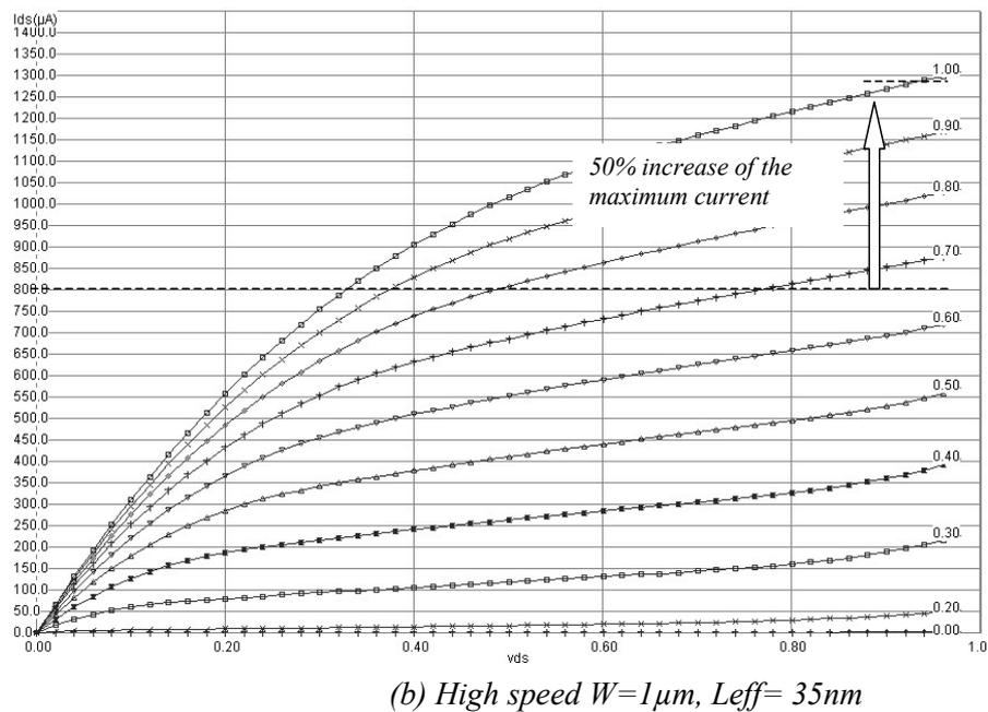
Figure 8:  $I_d/V_d$  characteristics of the Low leakage and high speed nMOS devices
