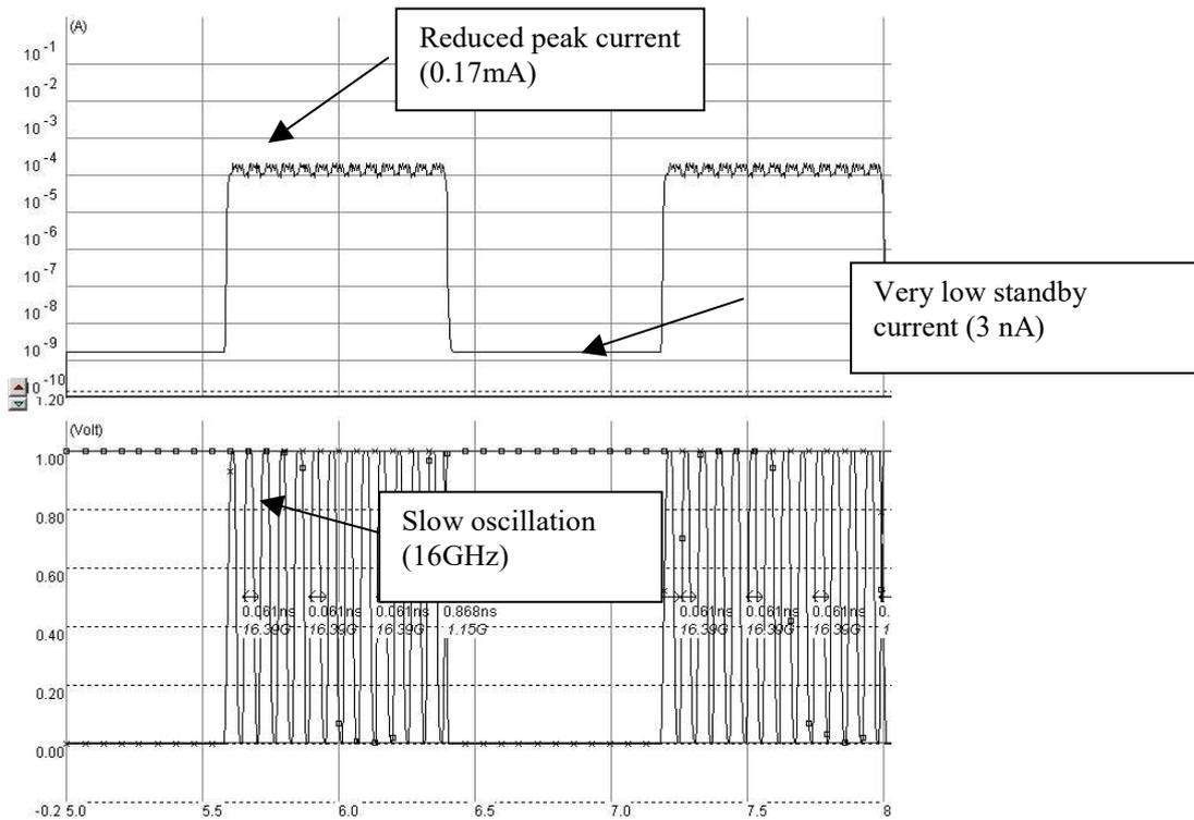
Figure 20: Simulation of the ring oscillator in low leakage mode. The oscillating frequency is slower but the standby current is very low (Inv5Enable.MSK)
