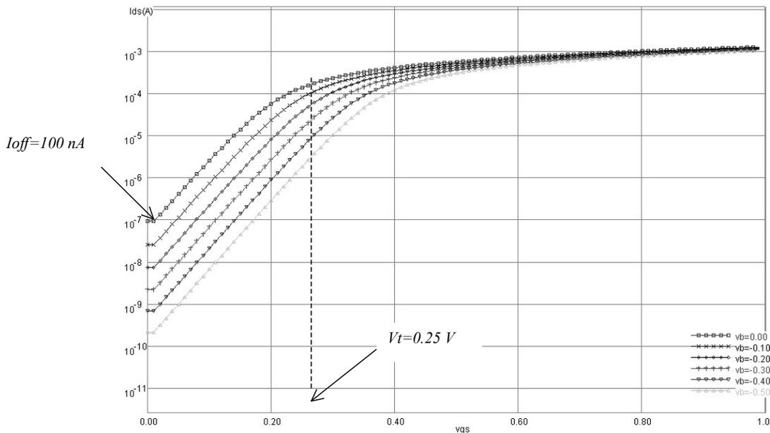
(b) *Id/Vg characteristics for high speed MOS ( $W=1 \mu m, L_{eff}=35 nm$ )*
