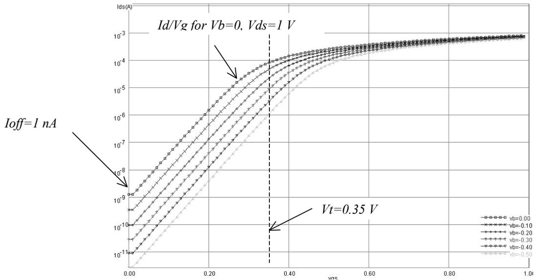
(a) *Id/Vg characteristics for low leakage MOS ( $W=1 \mu m, L_{eff}=50 nm$ )*
