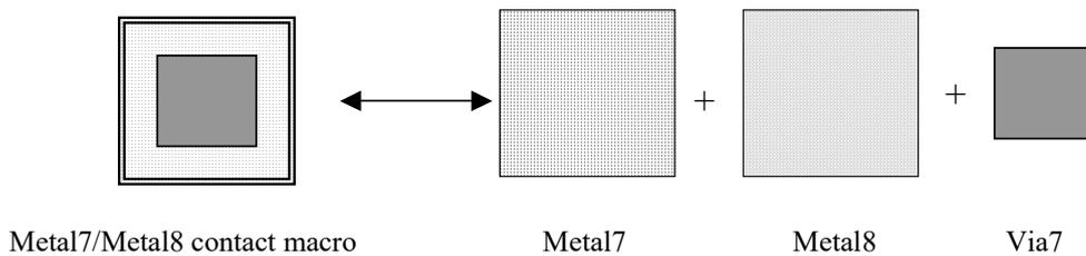
Figure 12: Access to contact macros between metal layers
