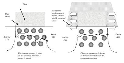
Figure 4: Tensile strain generated by a silicon-nitride capping layer increases the distance between atoms underneath the gate, which speeds up the electron mobility of n-channel MOS devices
