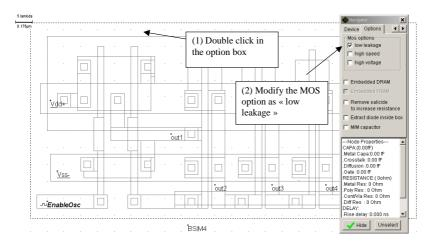
Figure 30: Changing the MOS option into low leakage mode
