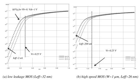
Figure 10: Id/Vg characteristics (log scale) of the low leakage and high-speed nMOS devices
