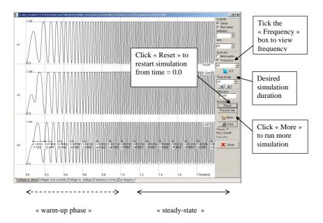
Figure 25: The simulation always starts by a "warm-up" phase (1.0 ns). Click "More" to run more simulation (Inverter > INV5.MSK)
