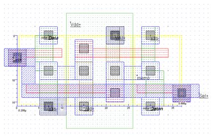
Figure 32: The 6-transistor RAM layout using 32-nm design rules (Ram6T\_32nm.MSK)
