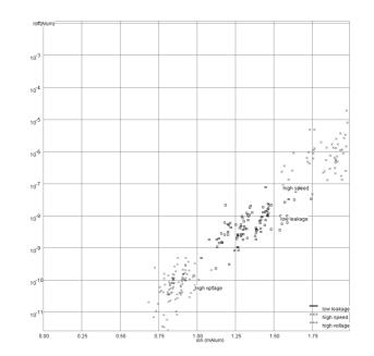
Figure 12: Ioff/Ion calculated by Microwind on 100 samples of n-channel MOS with random distribution of VT, U0, and LINT with a Gaussian distribution around the nominal value
