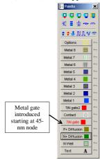
Figure 14: Microwind window with the palette of layers including 8 levels of metallization
