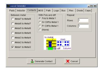
Figure 16: Access to complex contact generator
