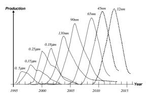
Figure 2 : Technology ramping every two years introducing the 32 nm technology
