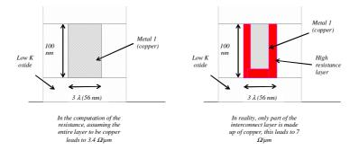
Figure 21: In reality, the lower metal layers feature a higher resistance, because the entire layer is not made up of low-resistivity material
