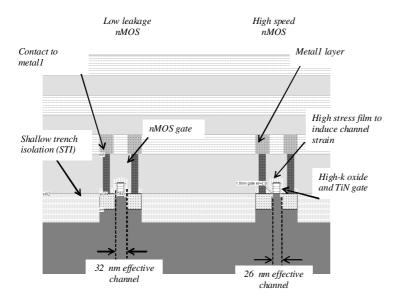
Figure 8: Cross-section of the nMOS devices (Mos/allMosDevices.MSK)
