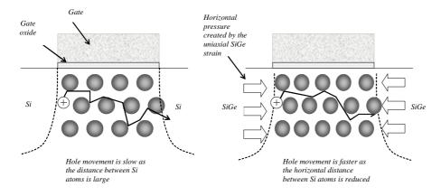
Figure 5: Compressive strain to reduce the distance between atoms underneath the gate, which speeds up the hole mobility of p-channel MOS devices
