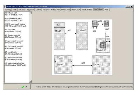
Figure 18: The Help > Design Rules menu of Microwind 3.5 gives details of the most important design rules
