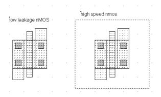
Figure 7: Layout of the low-leakage and high-speed MOS devices (Mos/allMosDevices.MSK). Dimensions are identical (2 lambda length).
