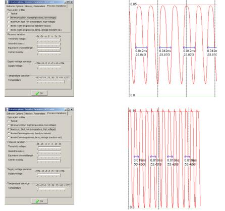
Figure 31: PVT Min-Max simulation showing 100% variation in switching performances
