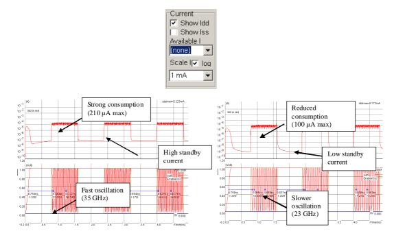
Figure 29: Simulation of the ring oscillator in high speed mode (left) and low leakage mode (right). The oscillating frequency is higher in high-speed mode but the standby current is also high (Inv5Enable.MSK)
