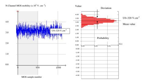
Figure 11: The extracted mobility of 1000 MOS samples shows an important variability around 320 V.cm<sup>2</sup>
