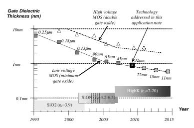
Figure 1 : The technology scale down towards nano-scale devices
