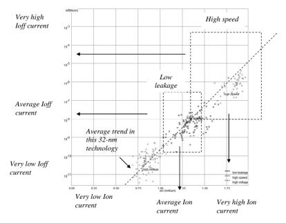
Figure 13: Finding compromises between high current drive and high leakage current
