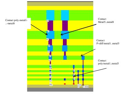
Figure 17: Examples of layer connection using the complex contact command from Microwind (Interconnects /Contacts.MSK)
