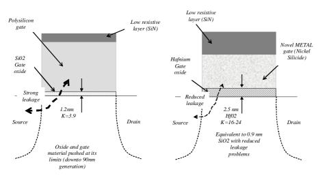
Figure 3: The metal gate combined with High-K oxide material enhances the MOS device performance in terms of switching speed and significantly reduces the leakage
