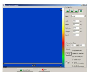
Figure 23: Realistic setup for evaluating metal2 total capacitance
