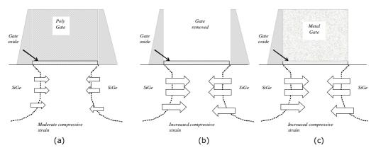
Figure 6: Increased p-channel MOS strain using a sacrificed poly gate and replacing it by metal gate [Natarajan2008]
