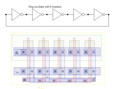
Figure 24: Schematic diagram and layout of the ring oscillator used for simulation (INV5.MSK)
