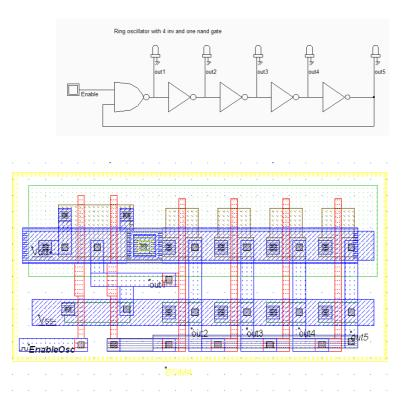
Figure 28: The schematic diagram and layout of the ring oscillator used to compare the analog performances in high speed and low leakage modes (INV5Enable.MSK)
