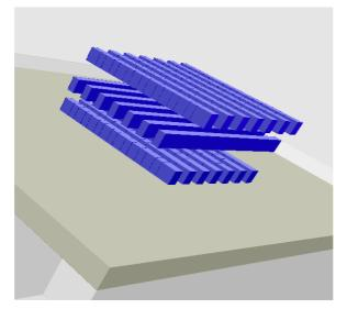
Figure 22: The interconnect capacitance is evaluated assuming that multiple wires are running below and above the layer under consideration (Interconnects > Metal1-3.MSK)
