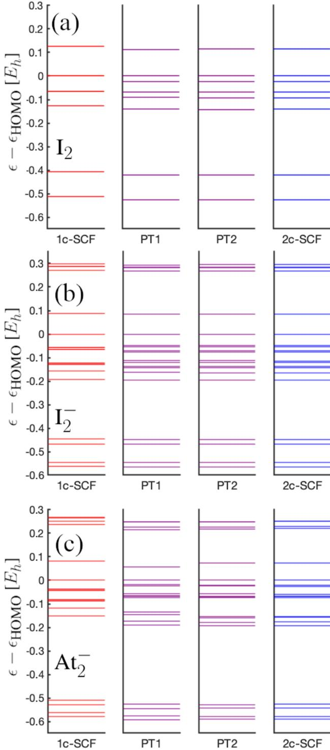
FIG. 2: KS eigenvalue spectrum calculated with the energy-consistent RECPs and PBE0 functional for  $\text{I}_2$ ,  $\text{I}_2^-$  and  $\text{At}_2^-$ . The eigenvalues are provided also in Tables S6-S8 of the ESI.
