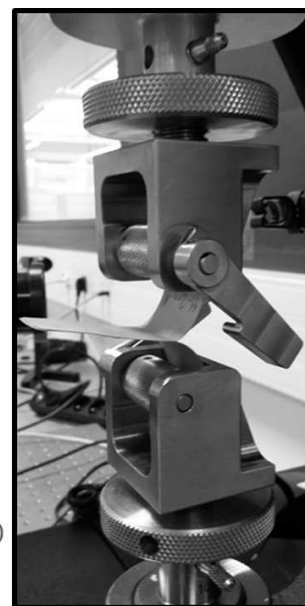
Figure 4. Peeling set-up to evaluate the performances of welded papers (right) and typical peeling curves of S1-S1 papers (left).
