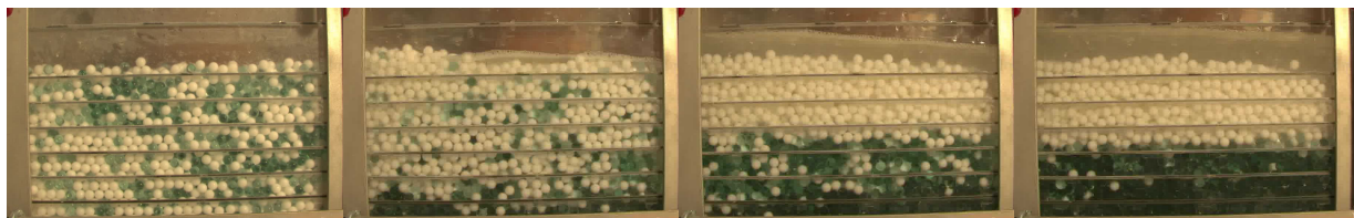
Figure 2: Evolution of the density sorting of glass and plastic beads that were (top) initially inversely sorted and (bottom) mixed. A cycle is constituted of a resuspension phase and a settling phase.
