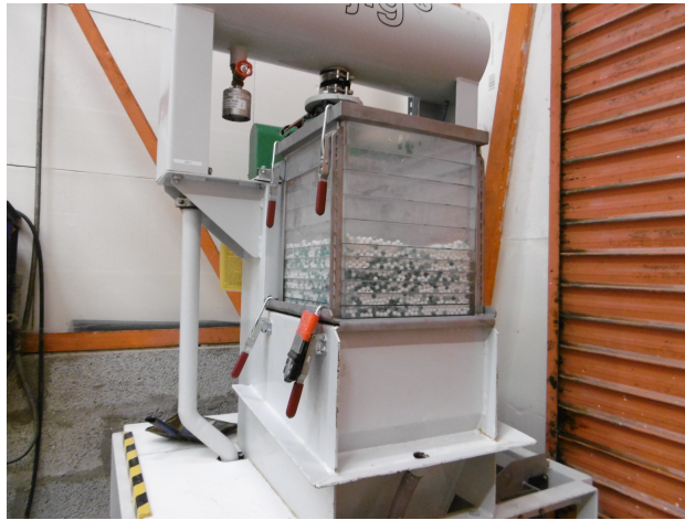
Figure 1: The experimental apparatus: a laboratory scale water jig (Allmineral Alljig).
