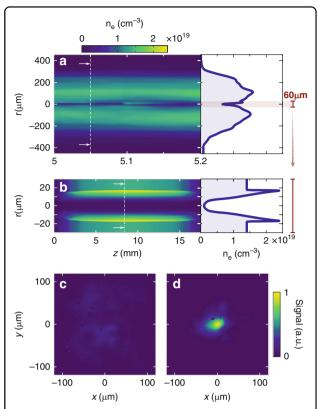
**Fig. 2 Plasma channel and guiding. a** Measured density profile. The density in the middle of the waveguide is overestimated because of limited resolution. **b** Simulated plasma channel (see Methods). **c**, **d**, Laser focal spot of P1, measured after attenuation of the full energy beam at the exit of the plasma, without (**c**) and with (**d**) guiding
