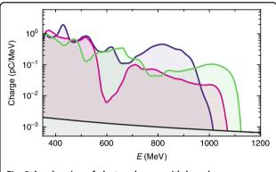
Fig. 3 Acceleration of electron beams with broad energy distributions. Three consecutive electron spectra obtained using ionization injection. The black line indicates the detection threshold.
