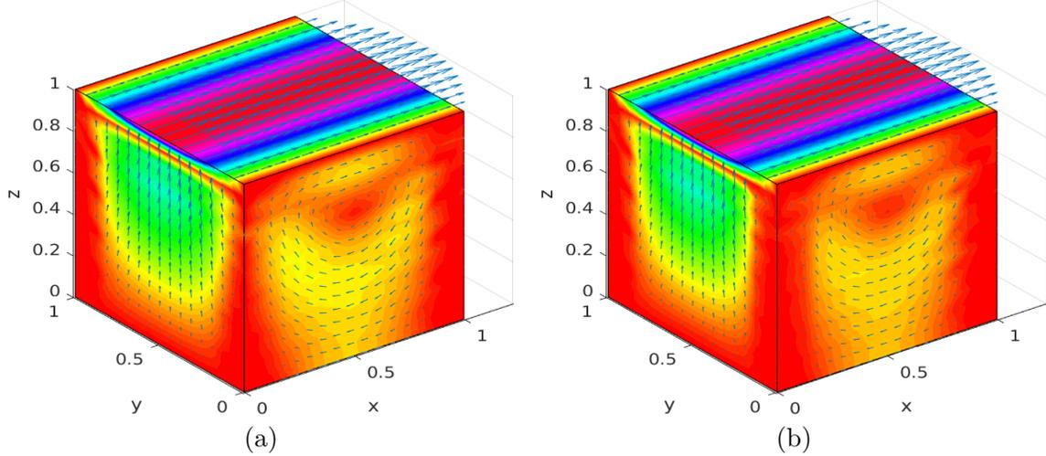
Figure 3: Velocity field and  $\| \mathbf{u}_\tau \|$  for the 3D lid-driven cavity (a):  $g = 0.25$ , (b):  $g = 2$
