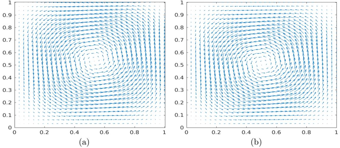
Figure 1: Velocity fields for the driven cavity problem (a):  $g = 0.25$ , (b):  $g = 1$
