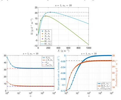
Figure 7: Up: First-two elements of these two sequences. Down Left: Surface biomass  $X_nh_n$  and optical depth  $\varepsilon(X_n)h_n$  for the sequence  $(X_n,h_n)_{n>0}$ . Down Right: Productivity  $\Pi(X_n,h_n)$  and net growth rate at the reactor bottom  $\mu(X_n,h_n)-R$  for the sequence  $(X_n,h_n)_{n>0}$ .
