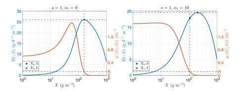
Figure 5: Productivity (II) with respect to biomass concentration (X) for  $h = 0.15 \,\mathrm{m}$ . Left:  $\alpha_1 = 0 \,\mathrm{m}^{-1}$ . Right:  $\alpha_1 = 10 \,\mathrm{m}^{-1}$ .
