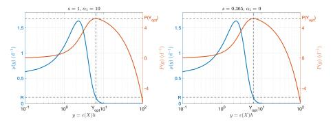
Figure 2: Growth rate  $\mu$  and optical depth productivity P with respect to y. Left: s=1 and  $\alpha_1=10\,\mathrm{m}^{-1}$ . Right: s=0.365 and  $\alpha_1=0\,\mathrm{m}^{-1}$ .
