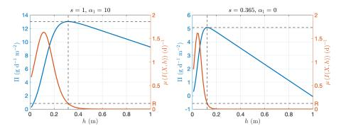
Figure 3: Productivity (II) and net growth rate  $(\mu_{\rm net}(X,h))$  with respect to depth (h) for  $X=50\,{\rm g\cdot m^{-3}}$ . Left: s=1 and  $\alpha_1=10\,{\rm m^{-1}}$ . Right: s=0.365 and  $\alpha_1=0\,{\rm m^{-1}}$ .
