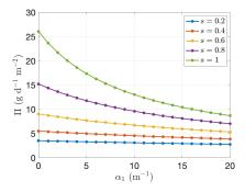
Figure 4: Optimal surface biomass productivity with respect to the background turbidity  $\alpha_1$  for  $X = 50 \,\mathrm{g \cdot m^{-3}}$  and different value of s.
