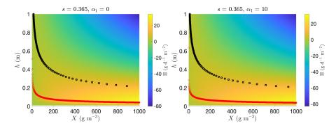
Figure 9: Global behaviour of productivity ( $\Pi$ ) with respect to depth (h) and biomass concentration (X). Left:  $\alpha_1 = 0 \,\mathrm{m}^{-1}$ . Right:  $\alpha_1 = 10 \,\mathrm{m}^{-1}$ . The red circles represent the suboptimal couple (X, h) where  $\Pi$  finds its maximum in the direction of h for a given X. The black squares represent the suboptimal couple (X, h) where  $\Pi$  finds its maximum in the direction of X for a given h.
