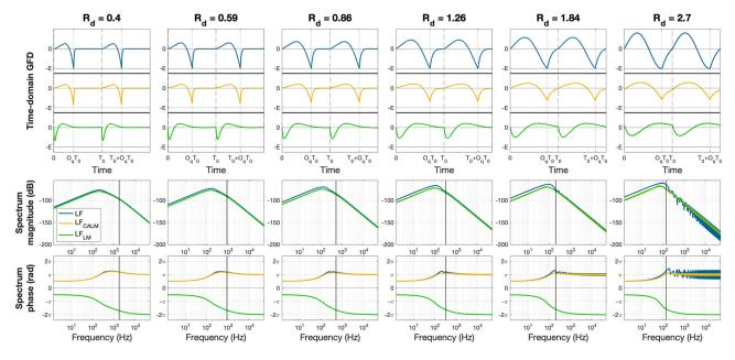
FIG. 5. (Color online) Glottal flow derivatives (top row) and their magnitude (second row) and phase (bottom row) spectra computed with the three models [LF (blue),  $LF_{CALM}$  (orange), and  $LF_{LM}$  (green)] for a range of  $R_d$  values (each column).
