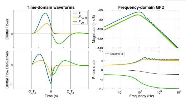
FIG. 3. (Color online) LF (blue),  $LF_{CALM}$  (orange), and  $LF_{LM}$  (green) waveforms including closed phases. Left: Glottal flows (top) and derivatives (bottom). Right: Magnitude (top) and phase (bottom) spectrum of the glottal flow derivatives.
