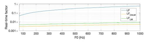
FIG. 4. (Color online) Computational efficiency of each model expressed in real-time factor: LF (blue),  $LF_{CALM}$  (orange), and  $LF_{LM}$  (green).
