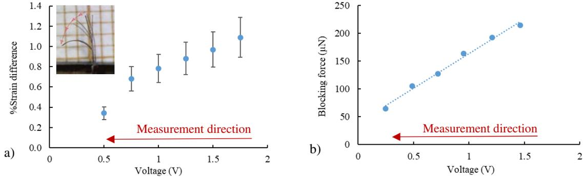
Figure 2: Measurements on one microbeam (width  $728 \mu\text{m}$ , thickness  $24.5 \mu\text{m}$ ) of an integrated PEDOT:PSS-based microtransducer. a) % strain difference and b) blocking force as a function of DC applied voltage from 1.5 to 0.25 V (error bars are smaller than the point size). In insert: microbeam embedded in SU-8 actuated with a  $V_{in}$  of 1.75 V applied on the remote gold contacts.
