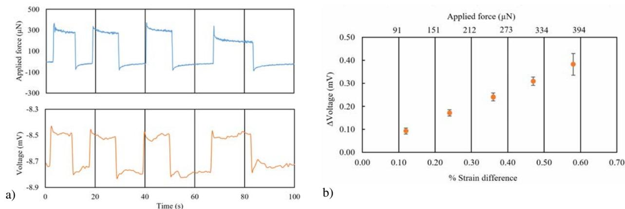
Figure 4: a) Force applied on a microbeam for a mechanical displacement of 500  $\mu\text{m}$  and the measured sensing voltage response. b) Sensing voltage ( $\Delta V$ ) as function of strain difference (%) or applied force ( $\mu\text{N}$ ). Measurement at 2 mm from the SU-8 encapsulation.
