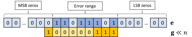
FIGURE 5. Illustration of the error range applied to CRC-CCITT-8 ( n = 8 ). Canceling LSB non-zero values by performing an XOR operation with a generator polynomial of width n + 1 bits produces an error range of n bits.
