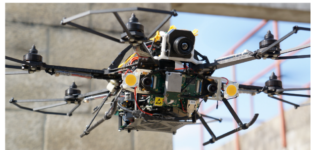
Figure 20: Firefly UAV equipped with the VI sensor [1].
