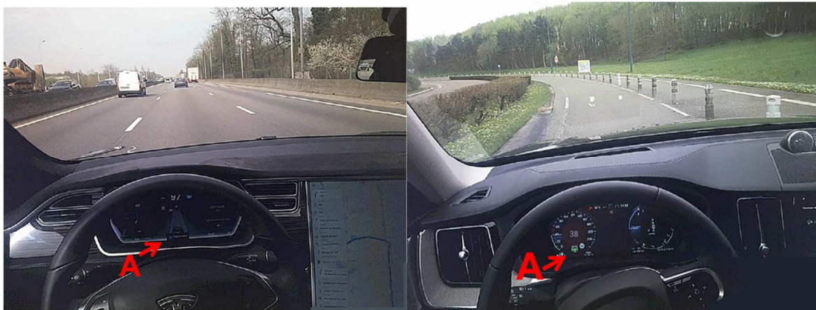
247 Figure 1: Photos showing the instrument panel and forward views of each vehicle with either 248 the driving-centered HMI (left) or vehicle-centered HMI (right). The letter A indicates the icon 249 displayed when LCA and ACC are activated.
