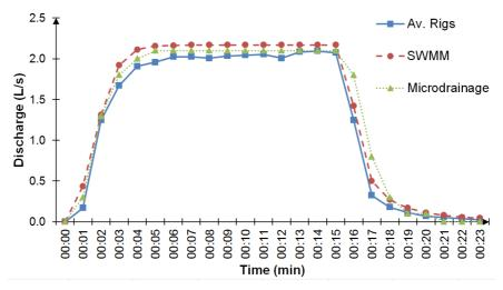
Figure 2. Hydrographs for the 10mm/h rainfall intensity and 15 minutes storm duration for a 100 m length HFD extrapolated from the results obtained for the laboratory models.
