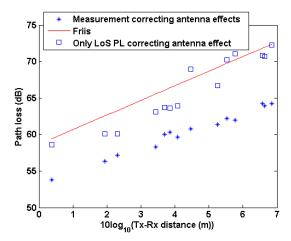
**Figure 5.** Measured path loss (PL) using all bandwidth, line-of-sight (LoS) PL, and Friis model. The antenna effect has been subtracted from the measured values.
