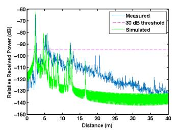
Figure 12. Comparison between the measured and simulated PDP for position number 10.
