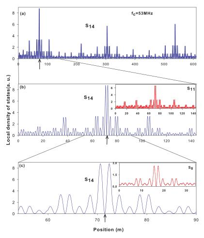
**Figure 4.** (**a**–**c**) Represent the spatial representation of the local density of states (LDOS) [in arbitrary units] of the mode lying at the central frequency  $f_c = 53$  MHz for the 14th generation. The insets of (**b**,**c**) correspond to the LDOS associated with the 11th and 8th generations at  $f_c$ , respectively.
