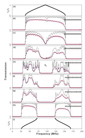
**Figure 2.** (**a**,**i**) Dispersion curves of the periodic structures composed of only B or only A blocks respectively. (**b**–**h**): Variation of the transmittance versus the frequency for different finite structures composed of 13 blocks *A* and *B*. (**e**) Transmission spectrum for generation  $S_6$  of the Fibonacci structure. The solid (dashed) curves represent the theoretical results with (without) dissipation, whereas open circles correspond to the experimental data.
