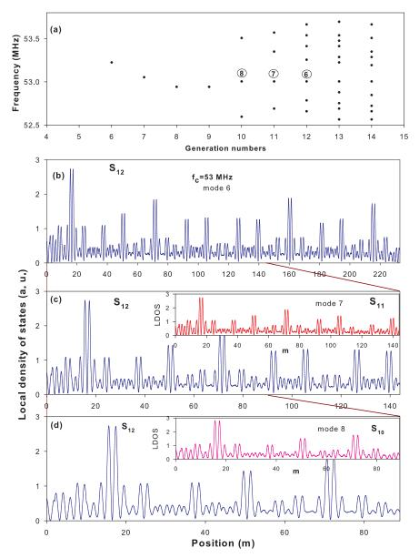
**Figure 9.** (a) Magnification of the FS modes around the central frequency  $f_c = 53$  MHz from Figure 7. (b–d) The LDOS (in arbitrary units) as a function of the space position *x* at the central frequency  $f_c$  for the 12th generation (mode 6) where the range on the horizontal axis is adapted for comparison to 11th and 10th FS generations. The insets of (c,d) correspond to the LDOS associated with modes 7 and 8 for the 11th and 10th generations at  $f_c$ , respectively.
