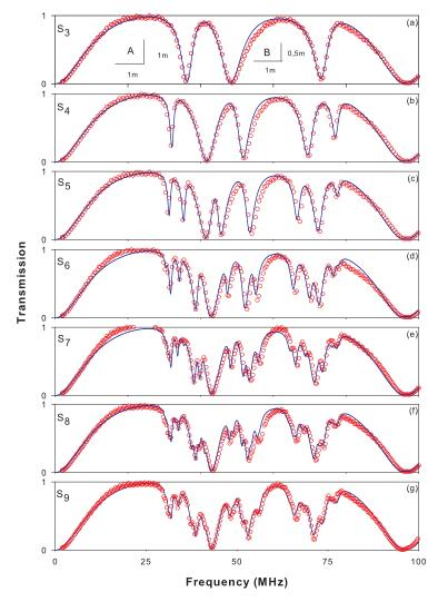
**Figure 6.** Theoretical (solid curves) and experimental (open circles) variations of the transmittance versus the frequency for a Fibonacci sequence inserted vertically along a waveguide (Figure 1g) for the generations  $S_3$ – $S_9$ .
