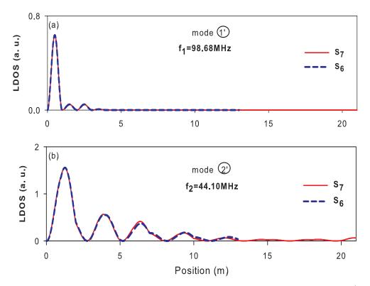
**Figure 11.** The LDOS (in arbitrary units) versus the space position *x* of the modes labeled 1' and 2' in Figure 10 at  $f_1 = 98.68$  MHz (**a**) and  $f_2 = 44.10$  MHz (**b**), respectively. Dashed (solid) curves correspond to the 6th (7th) generation.
