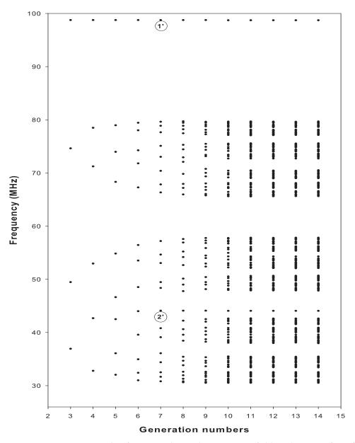
**Figure 10.** Same as in Figure 7 but for a FS with vanishing magnetic field on the top surface of the structure and vanishing electric field on the bottom surface. Here, the discrete modes are obtained from the minima of the transmission spectra displayed in Figure 6. The labels 1' and 2' correspond to the surface modes.
