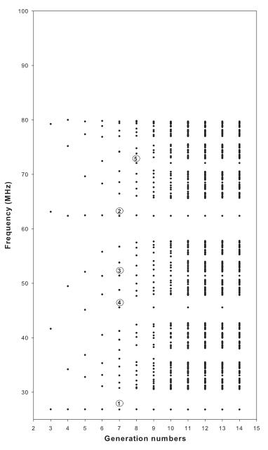
**Figure 7.** Dispersion of the eigenfrequencies (dots) of different generation numbers. The boundary conditions on both sides of the Fibonacci sequence (FS) are H = 0. One can notice the existence of primary and secondary gaps. All the discrete modes are obtained from the maxima of the transmission spectra displayed in Figure 6. The labels 1, 2, 3, 4 and 5 represent the surface modes.
