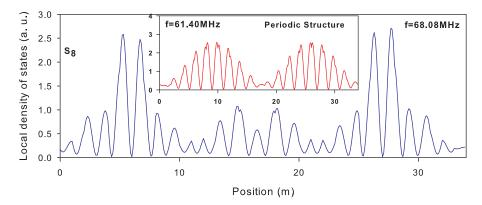
**Figure 5.** The local density of states (LDOS) [in arbitrary units] as a function of the space position x of the mode located at the band edge (f = 68.08 MHz) for the 8th generation. The inset of the figure corresponds to the LDOS associated with the periodic structure of length 34 m at f = 61.40 MHz.
