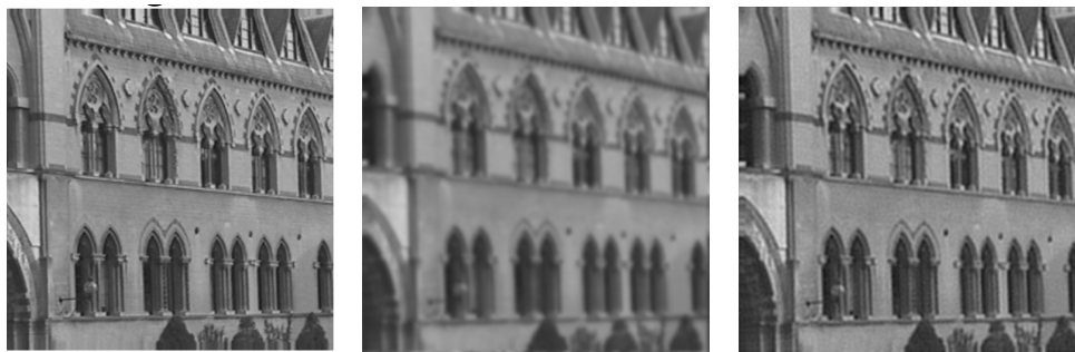
Figure 1.6: Example of image deblurring: image before degradation (left), degraded image (middle), deblurred image (right)
