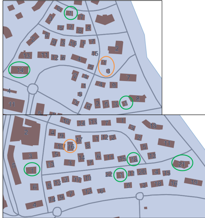
Figure 13: Multiple blocks with the elimination ordering computed with ELECTRE (1 means the first to be eliminated). Block delineations are displayed in blue, green highlights some good decisions, orange highlights questionable decisions.
