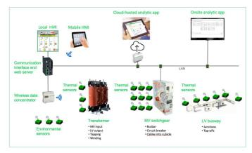
Figure 2. Continuous thermal monitoring architecture
