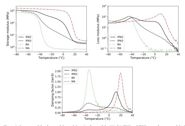
Figure 4: Storage modulus, loss modulus and damping factor of the MA, BA, IPN2 and IPN3 networks measured during torsion DMA temperature sweeps at  $2^{\circ}$ C/min.
