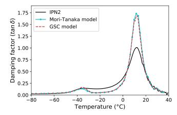
Figure 9: Comparison between IPN2 linear viscoelasticity and the Mori-Tanaka and generalized self-consistent estimates when the BA and MA input viscoelasticities have been shifted of +6 and  $-7^{\circ}$ C respectively.
