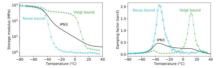
Figure 8: Voigt and Reuss bounds for IPN3 containing 70% of BA and 30% of MA when the MA input viscoelasticity have been shifted of  $-7^{\circ}$ C.
