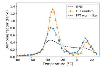
Figure 11: Comparison between the linear viscoelasticity of IPN3 and its representation by a worm-like and a random microstructure calculated by FFT-homogenization scheme when the MA viscoelasticity has been shifted of -7°C.
