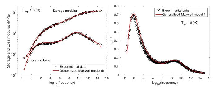
Figure 1: IPN1 shear storage and loss moduli and damping factor ( $\tan \delta$ ) master curves obtained by time-temperature superposition at reference temperature 10°C for torsion DMA frequency sweep tests. The solid lines show the fit of the experimental data by a generalized Maxwell model.
