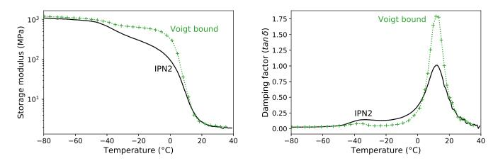
Figure 7: Voigt bound estimated for IPN2 when the BA and MA input viscoelasticity have been shifted of +6 and  $-7^{\circ}$ C respectively.
