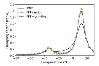
Figure 10: Comparison between the linear viscoelasticity of IPN2 and its representation by a worm-like and a random microstructure calculated by FFT-homogenization scheme when the BA and MA input viscoelasticities have been shifted of +6 and  $-7^{\circ}$ C respectively.
