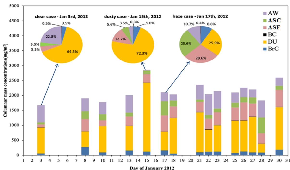
Figure 12. Time series of the daily mean of observed aerosol component mixtures, including BC, BrC, DU, ASF, SS, AW in Beijing region. The pie charts present the average aerosol component mixings for three episodes (clear, dusty and hazy) as marked in the figure.
