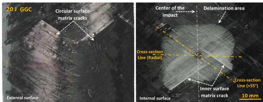
Fig. 18. Macro damage at GGC stacking hybrid composite pipe after low-velocity impact
