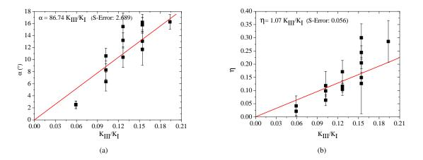
Figure 7: (a) The tilt angle  $\alpha$  is taken as the maximum value of  $\alpha(a)$  (blue dot in Fig.. 6b), the error bars corresponds to the standard deviation of the facet angle distribution at the peak location. (b) The coarsening rate  $\eta$  is taken as the slop of the linear part of the evolution d(a) (in blue in Fig.. 6c), the error bars corresponds to the upper and lower bounds of the 95 % confidence interval of the linear regression.
