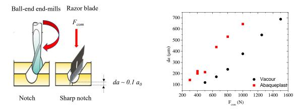
Figure B.10: Left: Notch milling and sharp notch formation. Right: Length of the additional precrack as a function of the compressive applied force for the two brands of PMMA (Vacour and Abaqueplast) used in this study.
