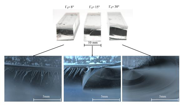
Figure 5: Fracture surfaces as observed by numerical microscopy.  $\Gamma_0 = 8^\circ$  corresponds to Type A, for  $\Gamma_0 = 15^\circ$  to Type C, for  $\Gamma_0 = 30^\circ$  to Type B.
