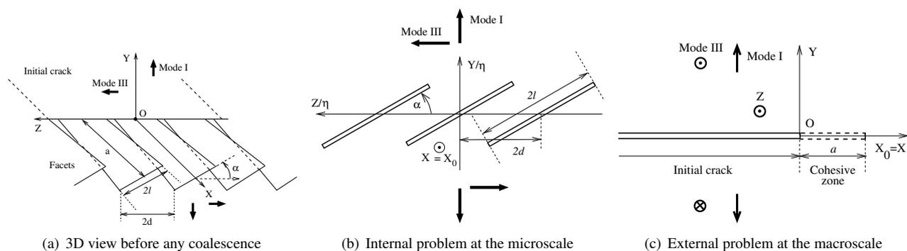
Figure 2: Sketch and notations of the initial crack and the facet formation: decomposition of the initial 3D problem (a) in two 2D problems: at the microscale (obtained by rescaling  $X$  and  $Y$  axis by  $X/\eta$  and  $Y/\eta$ , with  $\eta \equiv d/a \rightarrow 0$ ), the facets appear as an array of parallel echelon cracks subjected to remote stresses (b); at the macroscale, they are embedded in a cohesive zone (c).
