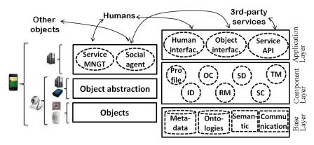
Figure 11. Architecture for SIoT: client side (left) and server side (right) (see [64]).
