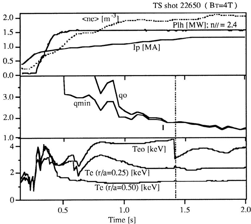
**Fig 1:** *Experimental scenario to perform the current profile in the current ramp-up phase with lower hybrid heating. The reversed shear configuration is maintained during almost 1s but terminates at 1.4s by a temperature collapse.*
