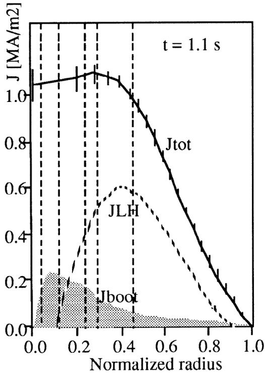
**Fig 2:** Total current and non-inductive currents calculated at 1.1s for the presented discharges. The location of the polarimeter chords are also indicated (--) as well as the variance inferred from the statistical analysis with IDENT-D.
