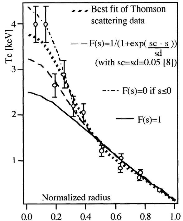
**Fig 4:** Simulation of  $T_e$  at 1.4s using the mixed Bohm/gyro-Bohm model and three different shear functions  $F(s)$  on the Bohm term.  $F(s) \neq 1$  seems required in the model to explain the measured temperature.
