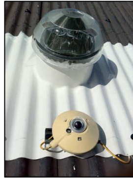
Figure 3: Outdoor pyranometer CMP11 for global irradiance in the plan of the light pipe
