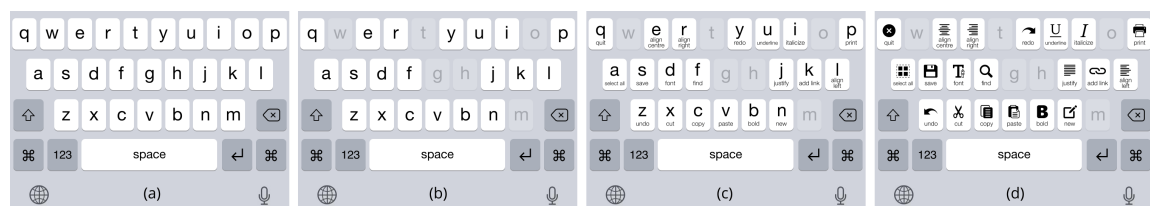
Fig. 2. Design variations for SoftCuts. (a) We modified the existing iOS keyboard by adding two command keys at the bottom row. (b) Design 1: Available shortcut keys retain their default appearance, while non-shortcut keys are greyed and inactive. (c) Design 2: In addition to Design 1, the name of each command is printed at the bottom of respective keys. Design 3: Similar to Design 2, but substituting the key labels with icons instead.
