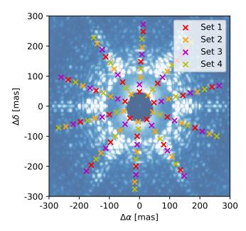
**Fig. 3.** View of the high-contrast images in the H configuration, with the position of injection of the companions overlaid. The companions are splitted in four different datasets to avoid the superposition of their PSFs. The dark asymmetric zone in the center is the focal plane mask, whereas the larger circular one is the zone optimized by the SP1 apodizer (see Carlotti et al. 2018 for details).
