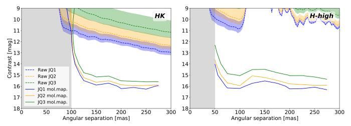
Fig. 8. Detection limits of the HARMONI high-contrast mode for the HK and H-high configurations and three different observing conditions. The dashed curves in the upper part of the plots show the raw HARMONI contrasts before any processing, with the envelope representing the  $1\sigma$  variance of the 120 exposures. The grayed-out part corresponds to the area masked by the anti-saturation focal plane mask.
