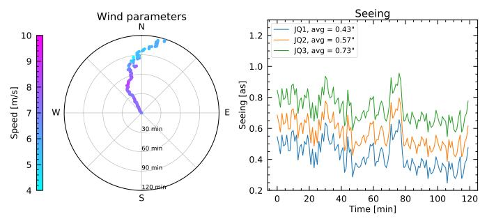
Fig. 1. Atmospheric conditions simulated for each exposure. The *left plot* provides the ground layer wind speed and direction and the *right plot* shows the seeing values for three different predefined conditions, which are labeled JQ1, JQ2, and JQ3 (see text for details).
