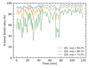
**Fig. 2.** Strehl ratio of the SCAO simulations averaged over the 2500 iterations of each HC exposure, for the three simulated seeing levels. Only atmospheric turbulence is simulated in the closed-loop sequences, additional telescope and instrument effects are separately added to the simulations.
