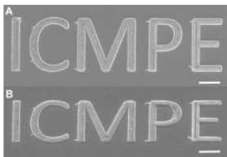
Figure 4. SEMs (A: Face image, B: 40° tilted image) of a microstructure fabricated by NIR induced polymerization of SOA resin with ACP (0.5 wt%, \lambda_{\text{irr}} : 800 nm, scale bar: 25 \mu\text{m} ).
