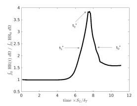
Figure 14: Time evolutions of I<sub>HR</sub> normalized by its initial value for the reference solution using the detailed chemical scheme GRI 3.0 [39].
