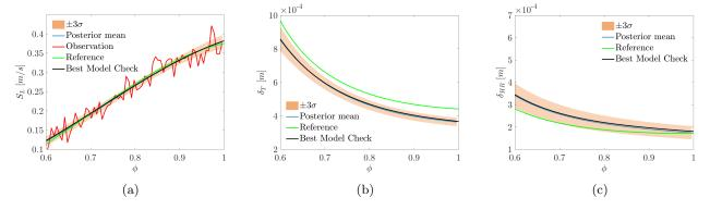
Figure 7: A posteriori predictions of (a) flame speed, (b) thermal flame thickness and (c) reaction zone thickness compared with the detailed kinetic mechanism (Reference). Case of the flame speed calibration.
