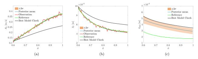
Figure 12: A posteriori results of (a) flame speed, (b) thermal flame thickness and (c) reaction zone thickness compared with the detailed kinetic mechanism (Reference) when the calibration is based on both the speed and the thickness of the flame, but considering a low value of  $\sigma_{\epsilon}$ .
