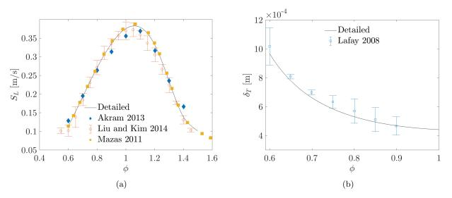
Figure 5: One-dimensional premixed flame results using GRI 3.0 [39] detailed chemistry. (a) Comparison of the computed flame speed with experimental results (Akram *et al.* [50], Liu and Kim [51]) and numerical (Mazas *et al.* [53]) studies. (b) Computed thermal flame thickness compared with experimental data of Lafay *et al.* [52].
