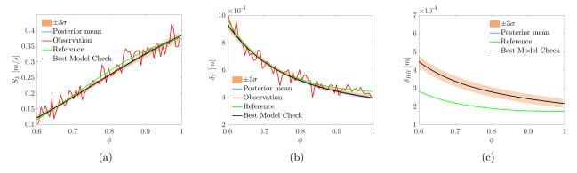
Figure 11: A posteriori results of (a) flame speed, (b) thermal flame thickness and (c) reaction zone thickness compared with the detailed kinetic mechanism (Reference) when calibration is based on both the flame speed and the thermal flame thickness.
