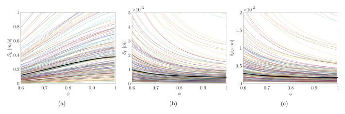
Figure 2: A priori QMC samples of the a priori global model as functions of the equivalence ratio  $\phi$ : (a) laminar flame speed, (b) laminar flame thermal thickness, and (c) laminar flame thickness based on heat release rate. The thick solid black line corresponds to the laminar flame speed and thicknesses for the detailed chemistry model discussed in § 3.
