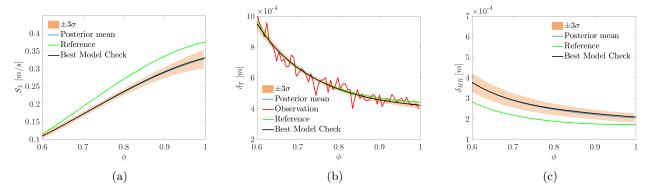
Figure 9: A posteriori predictions of (a) flame speed, (b) thermal flame thickness and (c) reaction zone thickness compared with the detailed kinetic mechanism (Reference). Case of the flame thickness calibration.
