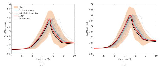
Figure 17: Time evolutions of the (a) normalized  $I_{HR}$  and (b) flame surface, for the calibrated two-step model. The time is normalized using the reference flame speed and thickness. The MAP and reference (using GRI 3.0 [39]) predictions are also reported.
