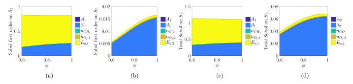
Figure 4: Sobol indices of first (a,b) and total (c,d) orders for the laminar flame speed, associated to the first (a,c) and second (b,d) chemical reaction parameters.
