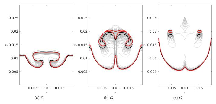
Figure 16: Progress variable isolines c = 0.5 at (a)  $t_1^*$ , (b)  $t_2^*$  and (c)  $t_3^*$ . Thin gray lines correspond to the samples of the reduced models, the black line refers to the detailed chemistry model, while the red line corresponds to MAP model.
