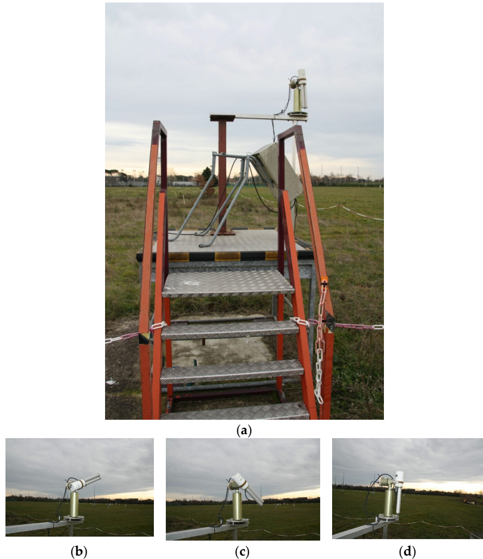
Figure 3. Toulouse sun/sky photometer: (a) pointing towards the sun; (b,c) rotating toward the surface; and (d) stand-by condition between two measurements.
