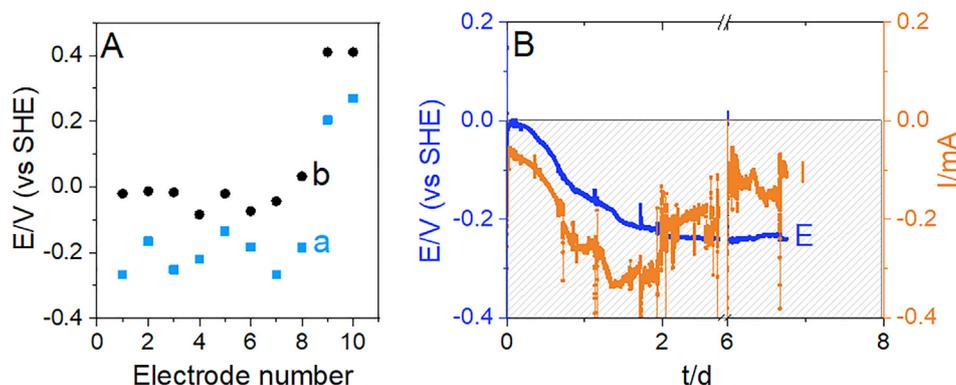
**Fig. 3.** (A) Open circuit potential of each electrode individually in absence of nitrate (a, blue squares) and presence of nitrate (b, black dots). The potential was measured 1 h after disconnecting electrodes from the whole snorkel. (B) Mixed potential of all electrodes connected in short-circuit (blue line) and current flowing between Electrodes #1–#8 (anodes – in sediment) and Electrodes #9&#10 (cathodes – in water) (orange line). Sediments from Rampillon.
