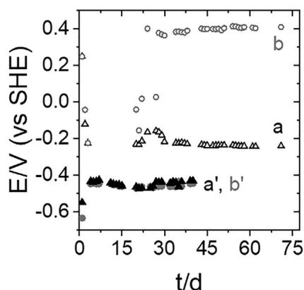
**Fig. 2.** Daily potential measurement with a MESs made of (a) graphite felt in sediment and metallic wire in water and (b) graphite felt in both sediment and water, connected together with a metallic wire. (a&b) were prepared with a stainless steel wire and (a'&b') with an iron wire. Sediments from Rampillon. Scheme of the experiment in Fig. S3 in Supplementary material.
