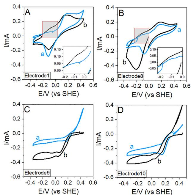
**Fig. 4.** Cyclic voltammetry of different electrodes in presence and absence of nitrate: (A) Electrode #1 (lowest position in sediment), (B) Electrode #8 (highest position in sediment), (C) Electrode #9 (lowest position in water) and (D) Electrode #10 (highest position in water). a (blue line) – without nitrate, b (black line) – with nitrate. Insets: zoom in the low potential region. Sediments from Rampillon.
