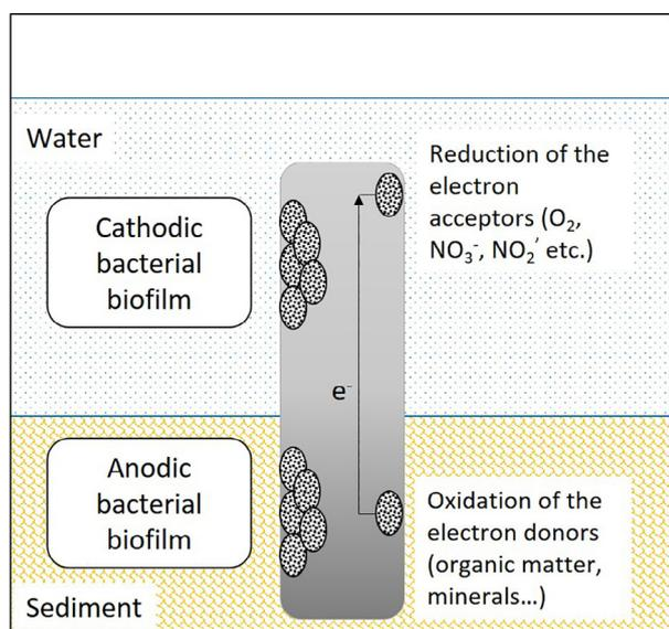
**Scheme 1.** Scheme of a Microbial Electrochemical Snorkel. The anodic bacterial biofilm oxidizes the electron donors present in the sediment. The electrons released in this process are collected by the Snorkel and transported to the part in water. Then, they can be used for the reduction of electron acceptors present in water by the cathodic bacterial biofilm.
