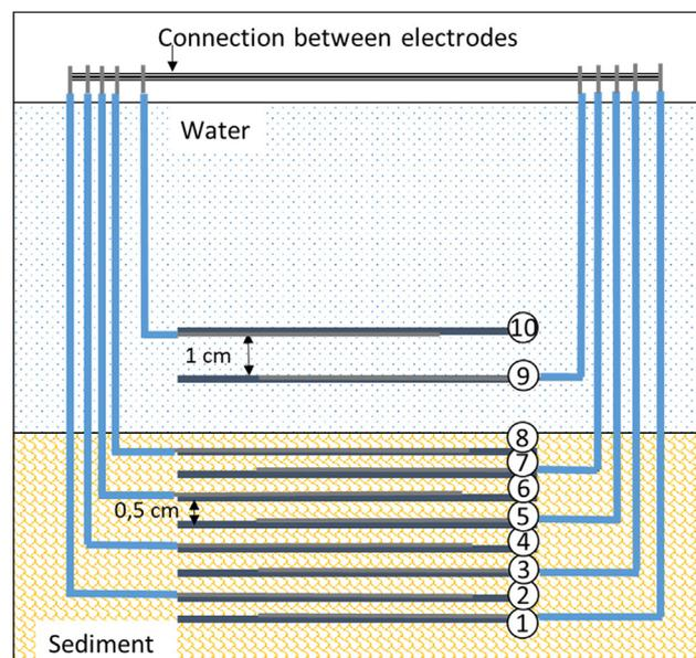
**Scheme 2.** Scheme of the Microbial Electrochemical Snorkel that was evaluated both in laboratory and *on-field*. The electrodes are numbered from the bottom (lowest Electrode #1, in sediment) to the top (highest Electrode #10, in water). The electrodes are made of stainless steel grid.
