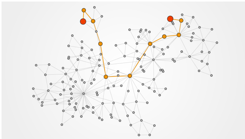
Figure 1: GraphStream algo core: shortest path computation
