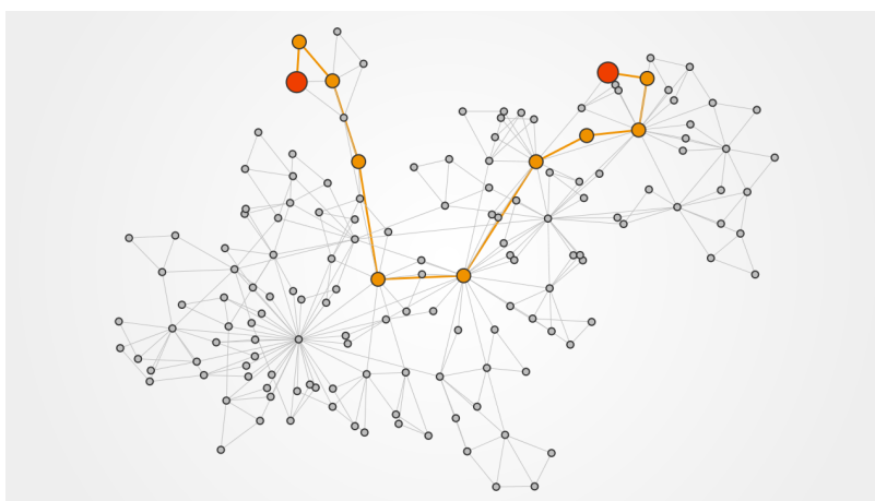
Figure 1: GraphStream algo core: shortest path computation
