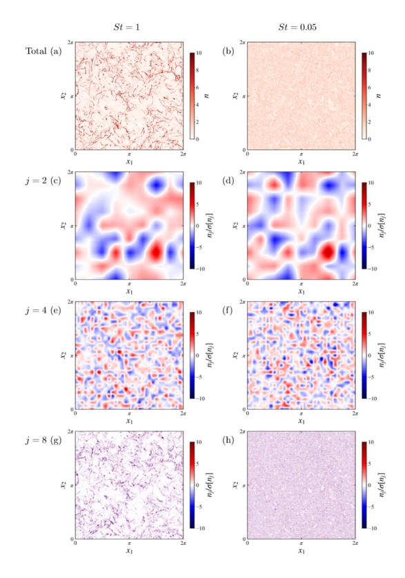
Figure 2. Spatial distributions of total number density field  $n(\mathbf{x})$  (a, b) and scale contributions  $n_j(\mathbf{x})$  at j = 2 (c, d), j = 4 (e, f) and j = 8 (g, h) in a  $x_1$ - $x_2$  cross section; (a, c, e, g) St = 1.0, (b, d, f, h) St = 0.05.
