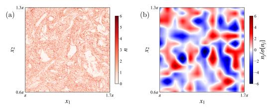
Figure 8. Magnified spatial distributions of (a) total number density  $n(\mathbf{x})$  and (b) scale contributions  $n_j(\mathbf{x})$  at j = 4 for St = 0.05 in the same  $x_1$ - $x_2$  cross section as Figure 2.
