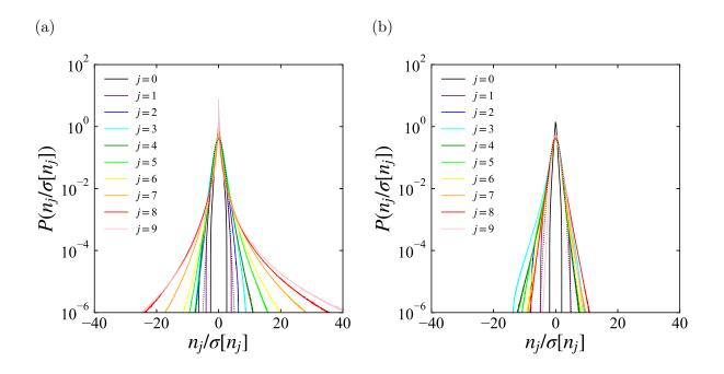
Figure 6. PDF of the normalized scale-dependent particle number density  $n_j/\sigma[n_j]$  for (a) St = 1.0and (b) St = 0.05 at  $Re_{\lambda} = 204$ . The dotted lines are the Gaussian distribution  $\mathcal{N}(0, 1)$ .
