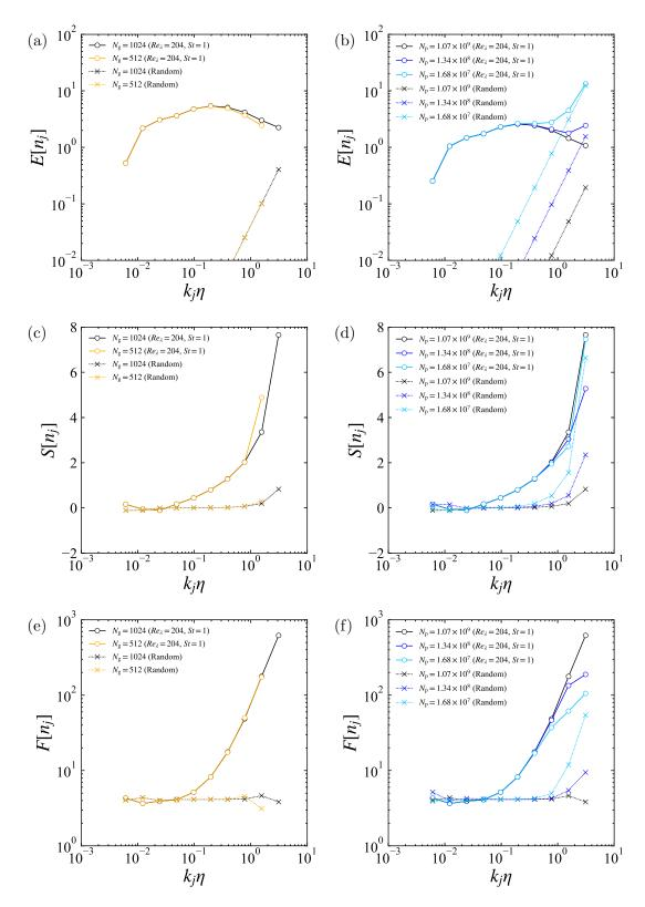
Figure 9. Wavelet spectra  $E[n_j]$  (a, b), scale-dependent skewness  $S[n_j]$  (c, d) and scale-dependent flatness  $F[n_j]$  (e, f) at  $Re_{\lambda} = 204$  and St = 1.0 for (a, c, e)  $N_g = 512$  and 1024 at fixed  $N_p(=$  $1.07 \times 10^9)$  and for (b, d, f)  $N_p = 1.68 \times 10^7$ ,  $1.34 \times 10^8$  and  $1.07 \times 10^9$  at fixed  $N_g(=1024)$ .
