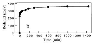
FIG. 2. Evolution of the FTIR transmission spectra (a) and the PL redshift (b), for a blue-green sample as a function of air exposure time.
