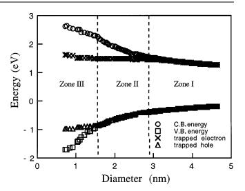
FIG. 3. Electronic states in Si nanocrystals as a function of cluster size and surface passivation. The trapped electron state is a *p*-state localized on the Si atom of the Si=O bond and the trapped hole state is a *p*-state localized on the oxygen atom.
