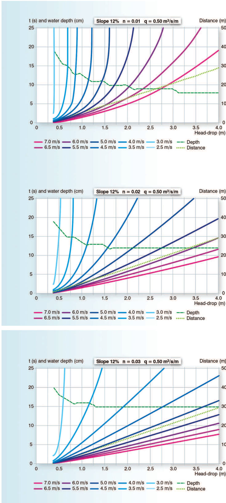
Passable head-drop (swimming) as a function of the maximum swimming speed U_{\text{max}} and the endurance t , for a discharge q = 0.5 \text{ m}^3/\text{s}/\text{m} and a constant slope of 12%. The three graphs correspond to three different roughness values ( n = 0.01 , n = 0.02 and n = 0.03 ). After Baudoin et al., 2014.
