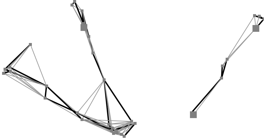
Fig. 4. A graphical view of a MANET. Black thick links are colored by the Spanning Forest Algorithm and belong to the forest. Bigger node are the ones owning a token , they are the roots or the spanning trees.
