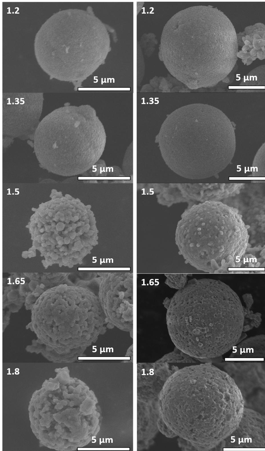
Fig. 6 : Li-rich NMC synthesized with different Li/M ratios at two different concentrations: 0.1 mol.L<sup>-1</sup> (left) and 0.4 mol.L<sup>-1</sup> (right).
