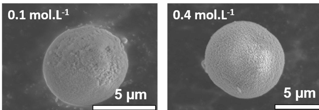
Fig. 4 : SEM images of the carbonate samples prepared at two concentrations, 0.1 mol.L<sup>-1</sup> and 0.4 mol.L<sup>-1</sup>.
