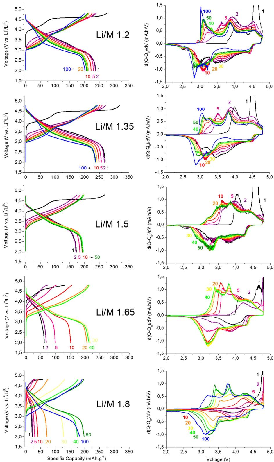
Fig. 9 : Galvanostatic charge-discharge curves of Li-rich NMC synthesized with different Li/M ratio (left) and respective  $dQ/dV$  plots (right).
