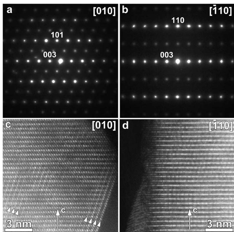
Fig. 13 : [010] (a) and  $[\bar{1}10]$  (b) ED patterns of the Li/M=1.35 material cycled 100 times (indexed in the trigonal basic cell of the O3 structure) and the corresponding [010] (c) and  $[\bar{1}10]$  (d) HAADF-STEM images (to be compared with the images of the pristine material in Fig. 11). The newly created  $\{10\bar{2}\}$  M-cation planes are marked with arrowheads.
