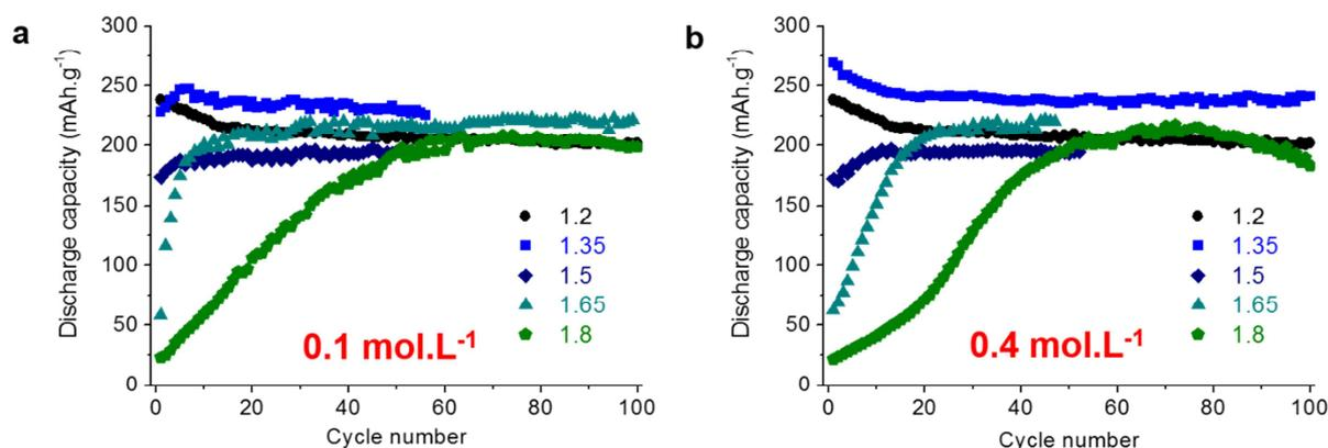
Fig. 10 : Capacity retention curves of Li-rich NMC synthesized with different Li/M at two concentrations, 0.1 mol.L<sup>-1</sup> (a) and 0.4 mol.L<sup>-1</sup> (b).
