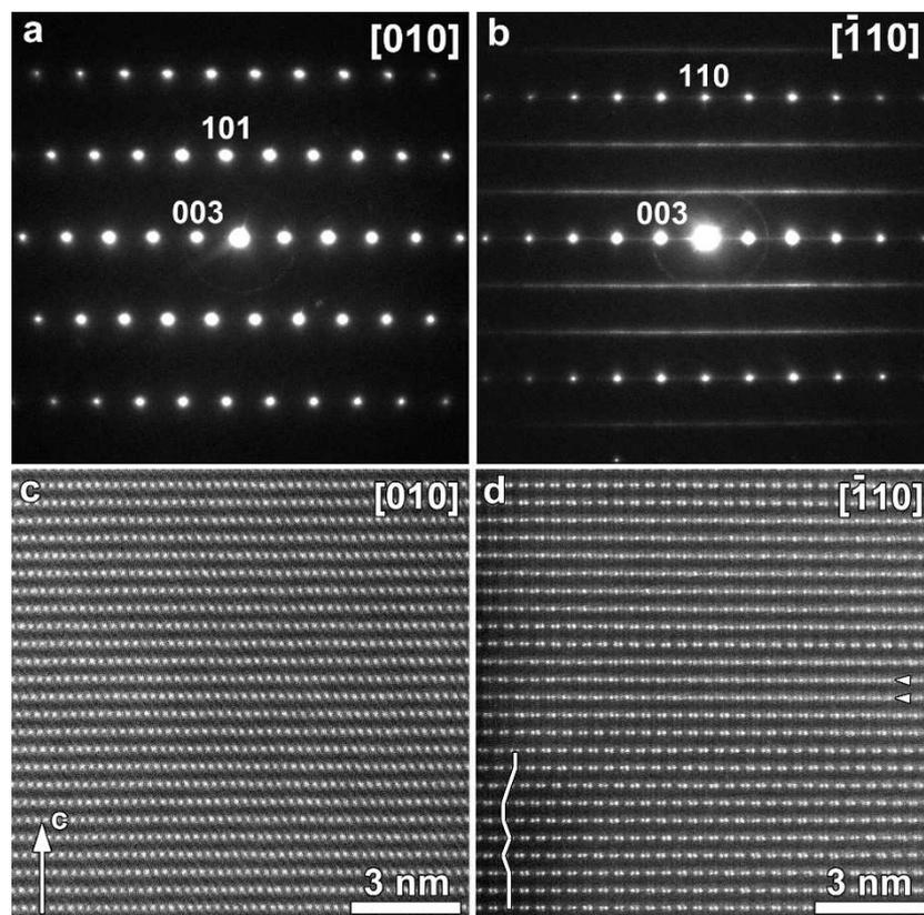
Fig. 11: [010] (a) and  $[\bar{1}10]$  (b) ED patterns of the pristine Li/M=1.35 material (indexed in the trigonal basic cell of the O3 structure) and the corresponding [010] (c) and  $[\bar{1}10]$  (d) HAADF-STEM images. The periodicity along the stacking direction of the “honeycomb” layers is violated by numerous stacking faults visible as lateral shifts of the  $\text{LiM}_2$  layers (traced with the white line). Some disordered  $\text{LiM}_2$  layers are marked with arrowheads.
