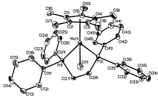
FIGURE 7. X-ray structure of Cp\*MoCl(dppe). Reprinted from ref 48. Copyright 1996 American Chemical Society.
