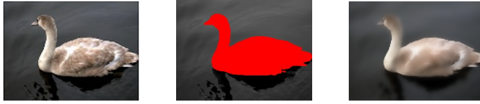
Fig. 2. Left: An image of dimensions 548 \times 402 from the Weizmann 1-object database [2]. Middle: Two labels are used to segment the pixels. The pixels belonging to the foreground are identified by the colour-code red. Right: The image on left is filtered using a bilateral filter [50]. A bilateral filter suppresses the texture details within objects which are irrelevant for summarizing the information on object boundaries in the image. The boundaries between the foreground and the background are crucial for image segmentation and are preserved.
