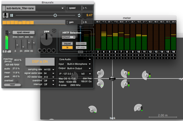
Figure 2. Binauralix GUI showing meterbridge and spat.viewer windows.
