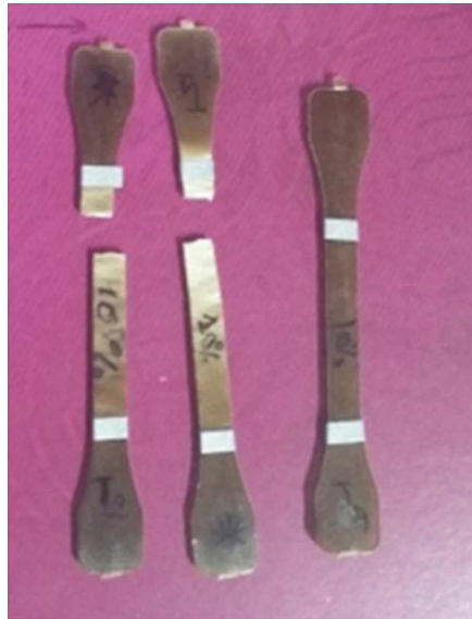
Fig. 6. Specimens before and after rupture.
