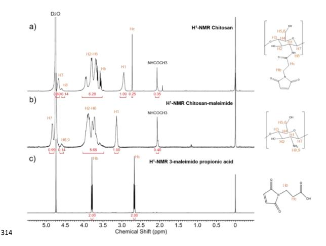
**Fig. 2**: H<sup>1</sup>-NMR (400 MHz, D<sub>2</sub>O) spectra and integration peaks of Chitosan-maleimide (**a**), Chitosan (**b**), 3-maleimidopropionic acid (**c**), and their respective chemical structures (right). All chemical shifts were expressed as  $\delta$  in parts per million (ppm), using the chemical shift of the residual solvent resonances as references (D<sub>2</sub>O:  $\delta$  = 4.80 ppm).
