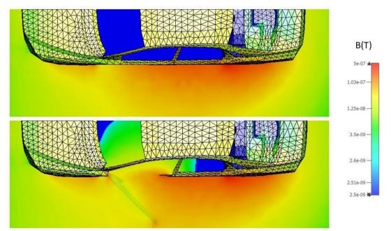
Figure 13. Effect of the door opening on the magnetic field levels (with Rx coil in central position below the car body). The maps of the B-field amplitude are reported at the height z = 0.4 m from the ground: (a) with closed door, (b) with open door [33].
