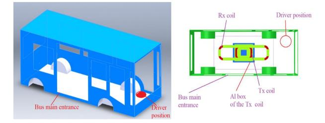
Figure 16. Bus body: a) 3D representation, b) plan view. The Tx coil size is  $0.8 \text{ m} \times 0.6 \text{ m}$  and the onboard Rx coil is  $2.5 \text{ m} \times 0.6 \text{ m}$ . The total length of the bus is 5.1 m, while the total width is 2.3 m.
