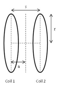
Figure 8. The arrangement of Helmholtz coils.
