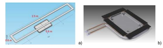
Figure 3. a) Bus Tx and Rx WPT coils (isometric view) and b) Tx 3D CAD design.
