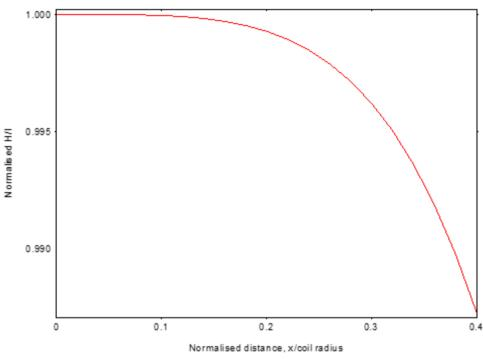
Figure 10. Variation of H/I across the central plane (X = 0) between the coils.
