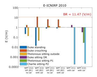
Figure 15. Peak of the E-field (V/m) averaged according to ICNIRP 2010 guidelines induced in the ViP phantoms. The horizontal red line represents the basic restriction (BR) level for induced E-field at 85 kHz according to ICNIRP 2010.
