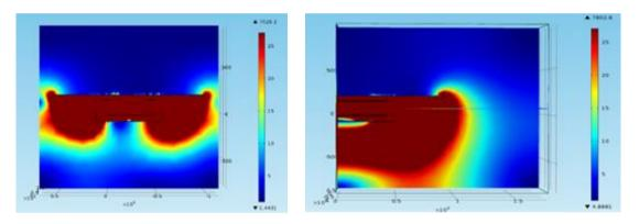
Figure A4. Magnetic field distribution simulation of the emitting and receiving WPT coils. Front and side views.
