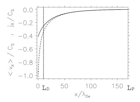
**Fig. 5:** Mean ion velocity  $v_x$  (dashed line) and current  $j_x$  (solid line) normalized to the sound speed  $c_s$  (no magnetic field).  $L_D$ : entrance of Debye sheath;  $L_P$ : bulk plasma.
