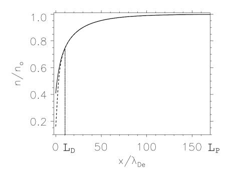
**Fig. 2:** Ion (solid line) and electron (dashed line) densities normalized to the bulk plasma density  $n_0$  (no magnetic field).  $L_D$ : entrance of Debye sheath;  $L_P$ : bulk plasma.
