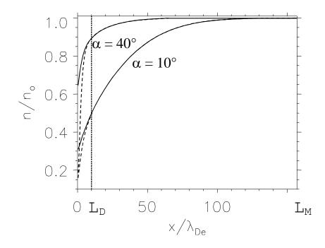
**Fig. 6:** Ion (solid line) and electron (dashed line) densities (normalized to the bulk plasma density) for different incidences of the magnetic field.  $L_D$ : entrance of Debye sheath;  $L_M$ : entrance of magnetic presheath.
