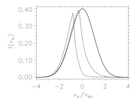
**Fig. 4:** Ion velocity distribution  $f(v_x)$  at x = 0 (wall, dotted line),  $x = 20 \lambda_{De}$  (intermediate position, dashed line) and  $x = 170 \lambda_{De}$  (Maxwellian bulk plasma, solid line). (No magnetic field).
