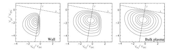
**Fig. 8:** Contours of constant level of the ion distribution in the  $(v_x, v_y)$  plane, at different positions, for  $\alpha = 10^{\circ}$ . (Dashed lines correspond to parallel and perpendicular axes to the magnetic field.) Left: x = 0, wall; middle:  $x = 26.6 \lambda_{De}$ , intermediate position; right:  $x = L_M$ , bulk plasma.
